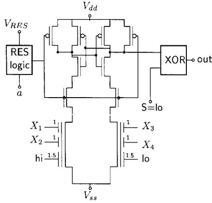
Fig. 7. Structure of the implemented logic block with neuron MOS threshold gate and additional boolean logic gates. In this example, the threshold function  $X_1 + X_2 > X_3 + X_4 + 1.5$  is shown.
