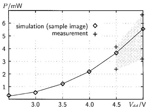
Fig. 11. Simulated and measured power dissipation at different supply voltages at a clock rate of 5 kHz (scaled to 40 000 PU's). Peripheral circuits are not considered.
