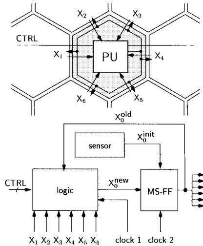
Fig. 5. Basic structure and input-output configuration of a PU with its six neighbors.
