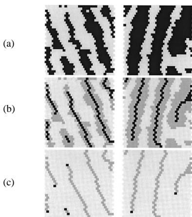
Fig. 12. Two typical measurement results: (a) sensed images, (b) their skeletons, and (c) the extracted ridge endings. In each image, the previous one is highlighted as a gray shadow.
