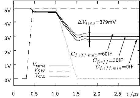
Fig. 4. Simulated  $V_{\text{sens}}(t)$  with  $C_{f,\text{eff}}$  as parameter ( $V_L = 5 \text{ V}$ ,  $\Delta V_{\text{CE}} = 5 \text{ V}$ ,  $C_{\text{CE}} = 105 \text{ fF}$ ,  $C_{\text{par}} = 121 \text{ fF}$ ).
