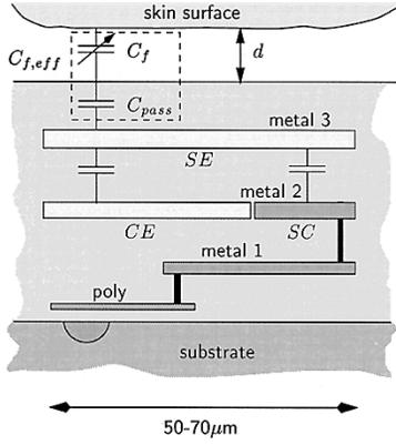
Fig. 2. Schematic cross section of a PU with the relevant parasitic capacitances of the sensor electrode. The circuits of the PU are wired with metal 1 and poly.
