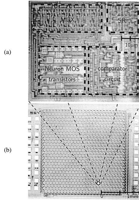
Fig. 10. Photograph of (a) a PU hidden below each hexagonal sensor electrode and (b) the demonstrator circuit.
