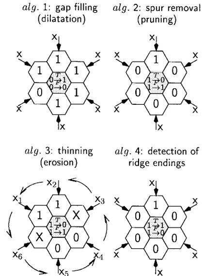
Fig. 6. Implemented structuring elements with boolean conditions for binary morphological image processing (T: true; F: false).
