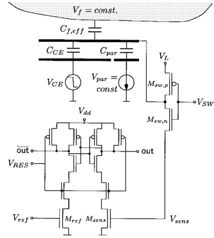
Fig. 3. Sensor circuit with dynamic latch as comparator for binarization of image data.
