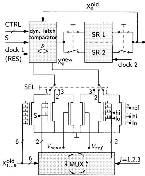
Fig. 8. Block diagram of the configurable PU ( $SEL = 1$ : Algorithms 1, 2, and 4;  $SEL = 2$ : Algorithm 3;  $SEL = 3$ : sensing process).
