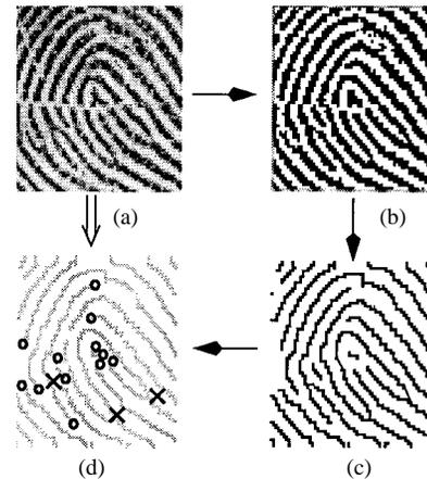
Fig. 1. Processing steps from (a) the sensed fingerprint image to (d) the extracted minutiae (o: ridge endings, x: ridge bifurcations). (a) Image acquisition, (b) binarization, (c) thinning, and (d) minutiae extraction.
