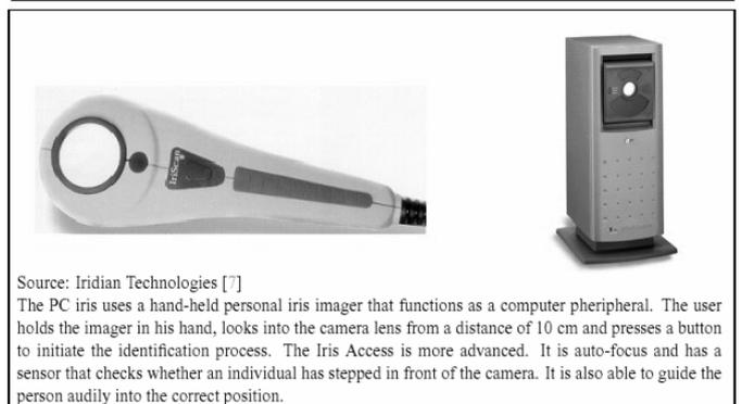
The iris scanner does not need any special lighting conditions or any special kind of light (unlike the infrared light needed for the retina scanning). If the
