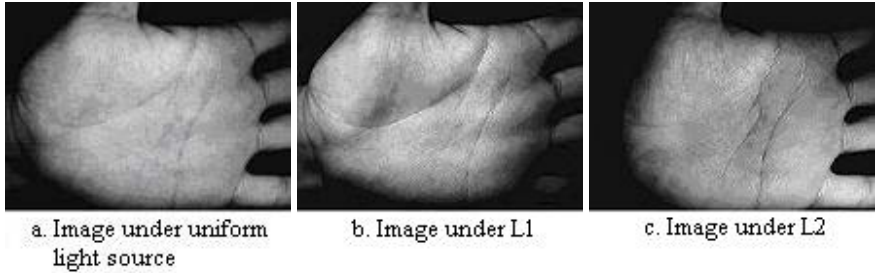
Fig. 8. Image under uniform light source and under the time-sharing light source
