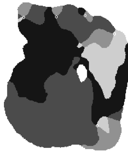
Fig. 4 Directional image of a palmprint (different gray levels represent different directions, and the center of each white circle corresponds with a delta point shown in Fig. 2).
